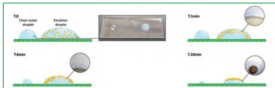
Figure 2: T.0 – Illustration of the evaporation process over ten minutes for a clean water droplet compared to an emulsion-containing droplet.
